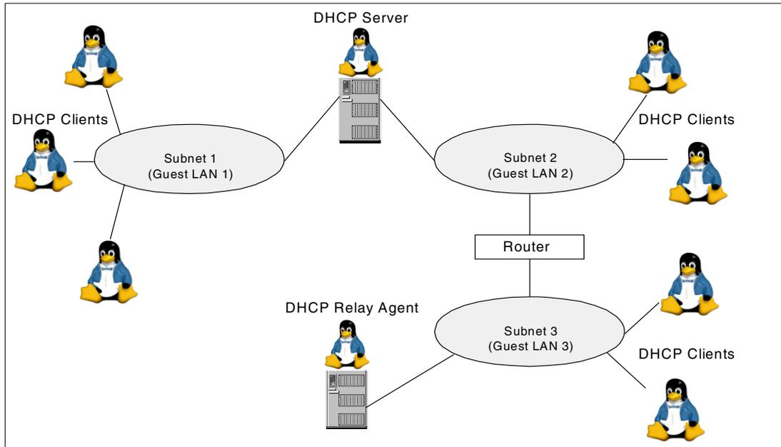
Figure 4 DHCP network components
